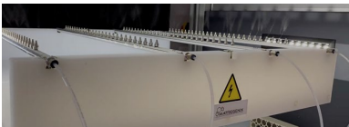
Close up of Matregenix R&D lab equipment creating new filters with electrospun nanofiber filters
